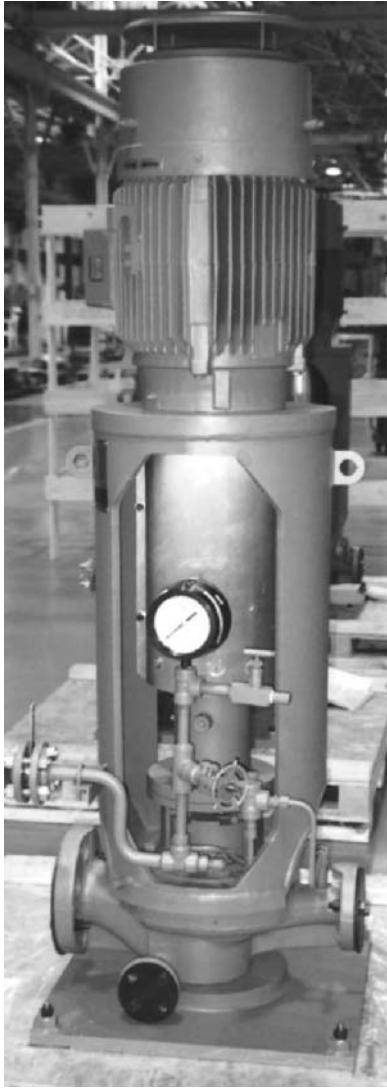
FIGURE 6 Single stage, overhung, vertical inline pump with separate bearing frame—API 610 Type OH3 (Flowserve Corporation)
