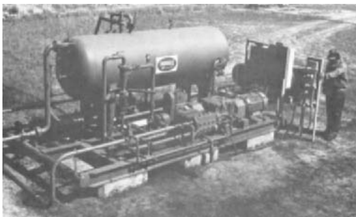
FIGURE 10 One-well unitized system (National Supply)
