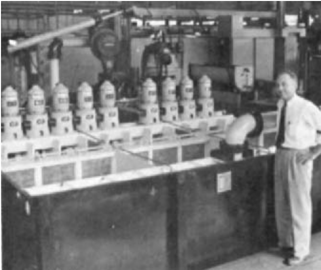
FIGURE 17 Model pit test setup with fixed screens and pumps and valves for variable flow, to scale (Flowsolve Corporation)
