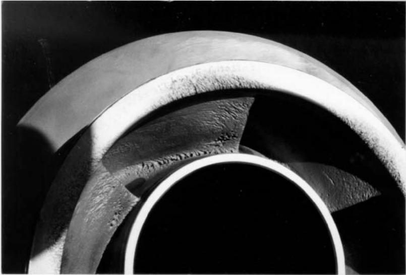
FIGURE 7 Cavitation erosion of an impeller, indicated by the porous appearance of cavitated regions on the surface
