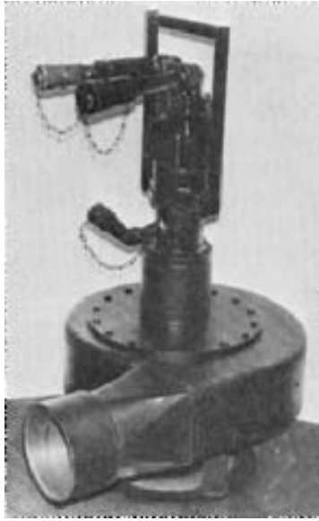
FIGURE 5 Portable centrifugal volute trash pump driven by hydraulic motor (M & W Pump)
