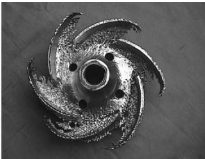
FIGURE 13 An austenitic stainless steel impeller in an abrasive fly ash service that shows severe erosion. Increased erosion occurs with an increasing fluid velocity near the periphery of the impeller.
